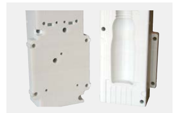
Figure 8: FDM blow molding tool made from polycarbonate.
