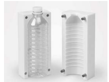
Figure 3: Blow mold constructed from the FDM process.
