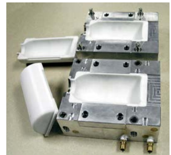
Figure 9: FDM hybrid tool with contoured inserts
