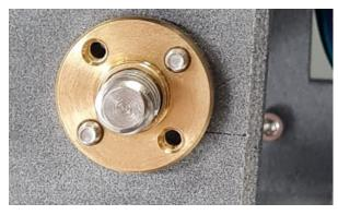
Lead screw nut bolt holes printed directly into the part. Slight misalignment of this part could cause issues in the operation of the lead screw, accuracy is critical making SAF<sup>TM</sup> PA12 the ideal material.
