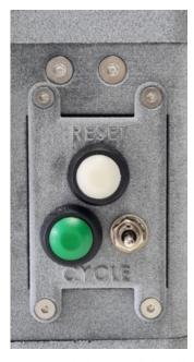
The fine feature resolution possible with the H350 and SAF™ PA12 allows for labels to be printed directly onto the part for clearly displaying the functions of buttons.
