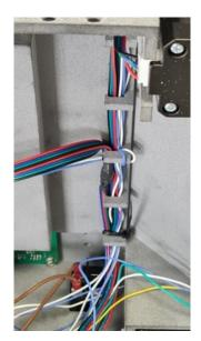
Design freedom of H350 and SAF technology allows for cable management to be printed directly onto the chassis, requiring no assembly after printing. Any modifications to the design in future can be made quickly and parts reprinted.
