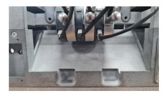
The measurements taken from the dogbone are fed instantaneously to the tensile testing software, ready for the dogbone to be pulled.
