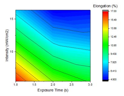
Printing parameters influence the degree of conversion and ultimately on part performance, in this case how modifying UV exposure intensity and time affects percent elongation.
