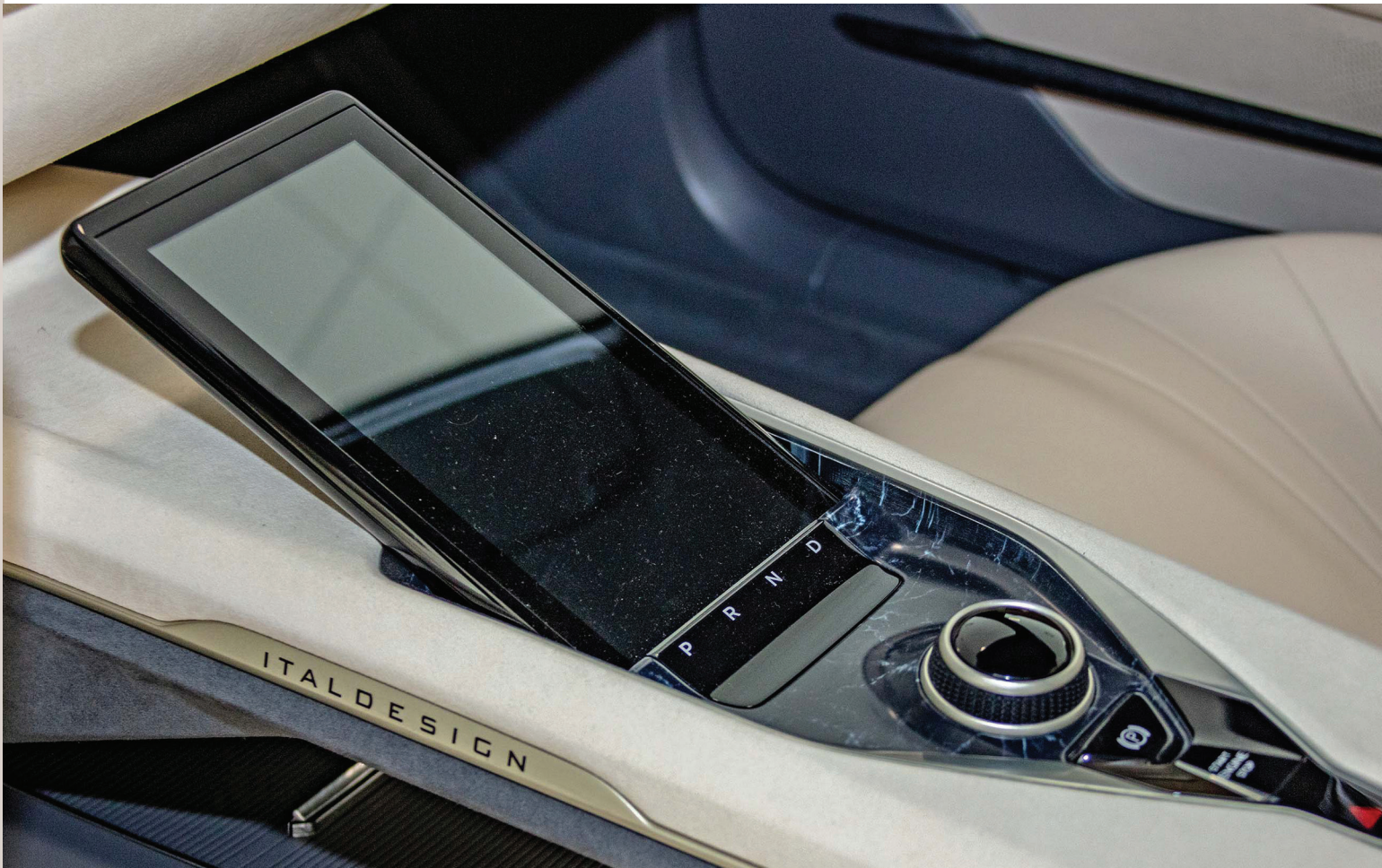
3D printed central console with marble effect.
