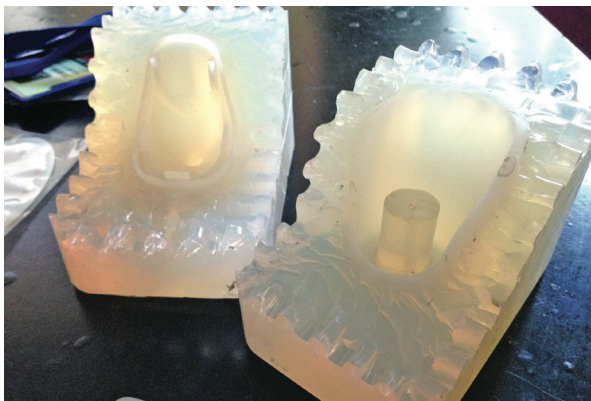
Solidify 3D printed a master part to create these silicon rubber molds for their automotive client.
